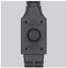
The on-screen menu is accessed and operated by the OSD control button shown. Simply depress the control button once to access the Main Menu then move the button up, down, left or right to navigate the options.
